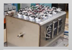
Transducer bonded in tank bottom, this technology may damage tank bottom after few years.
