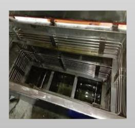
A vapor degreaser uses boiling solvent, rather than water, for fast precision cleaning and removal of true oils from parts. Vapor degreasing machines apply the principles of distillation and condensation to achieve high-quality cleaning and quick drying.
