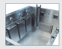
There are two basic ways to introduce ultrasonic energy into a cleaning tank. The first is to bond individual ultrasonic transducer elements directly to the exterior of a stainless steel tank. The second is by using submerged, liquid tight housings containing a number of transducer elements bonded internally and directed through the wall of the housing into the surrounding cleaning liquid.
